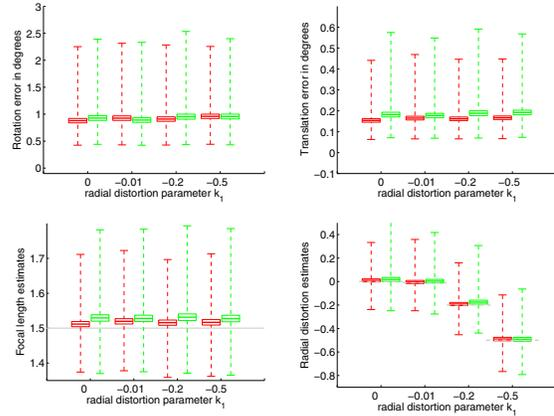
Figure 4. Error of rotation (Top left), error of translation (Top right), focal length estimates (Bottom left) and radial distortion estimates (Bottom right) in the presence of  $1px$  noise and different radial distortions for the new P5Pfr solver (Red) and the P4Pfr non-planar solver [5] (Green).
