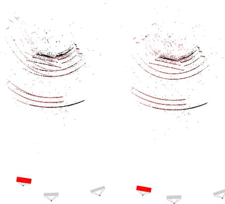
Figure 5. Camera registered using the P3P algorithm [8] and focal length extracted from *EXIF* (Left) and camera estimated using the new P5Pfr solver (Right). The black point cloud was calculated using gray cameras only. The red point cloud was created by triangulating 2D matches between red and gray cameras. Notice a strong misalignment in the P3P result (Left) caused by a small radial distortion present in the red camera.
