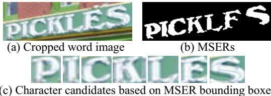
Figure 3: Character detection based on MSERs. For better illustration, only the non-overlapping MSERs are shown in (b). The handling of overlapping MSERs will be discussed later.
