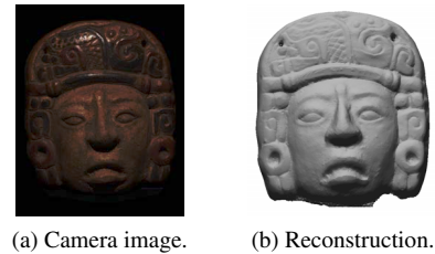
Figure 3: Results on a photometric stereo dataset: In particular, the painted regions of the clay mask exhibit specularities which leads to a violation of the assumption regarding Lambertian reflectance behaviour. Nevertheless, the reconstruction preserves the shape in these regions.
