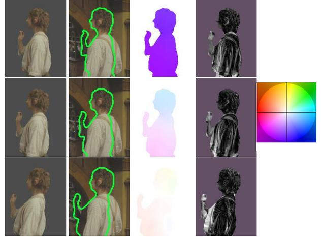
Figure 3: **Occlusion estimation and warping.** [Top to bottom]: Beginning ( $\tau = 0$ ), intermediate, and final stages of evolution. [1<sup>st</sup> column]: radiance  $a_\tau$ , [2<sup>nd</sup>]: target image  $I$  and boundary of  $R_\tau$ , [3<sup>rd</sup>]: velocity  $v_\tau$ , [4<sup>th</sup>]: occlusion estimation  $F^2$  at time  $\tau$ , [5<sup>th</sup>]: optical flow color code. The final occluded region is shown in Fig. 2(b).
