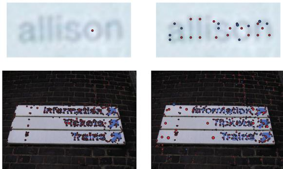
Figure 12: Keypoints detected by the FAST (left) and by the FASText detector (right). The size of the mark is proportional to the scale where the keypoint was detected.
