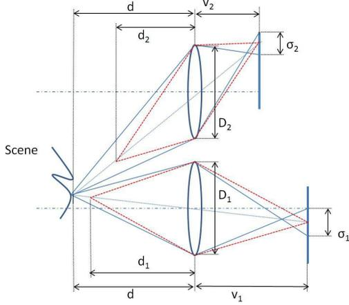
Figure 2: Optical geometry of defocus stereo based on thin lens model.
