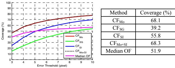
Figure 7: Performance of different methods of motion estimation along contours. **Left:** coverage score under different error threshold. **Right:** coverage score under error threshold 6.
