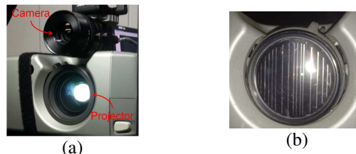
Figure 2. Actual optical system. (a) Setup with a short baseline and (b) coded aperture installed on the projector lens.
