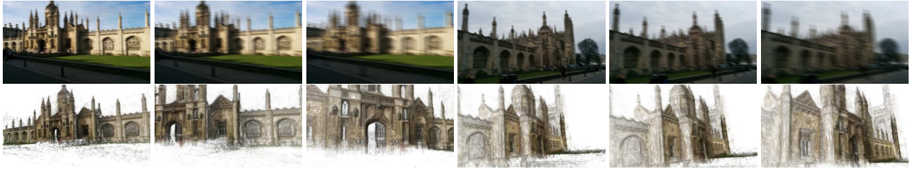
(a) Relocalization with increasing levels of motion blur. The system is able to recognize the pose as high level features such as the contour outline still exist. Blurring the landmark increases apparent contour size and the system believes it is closer.
