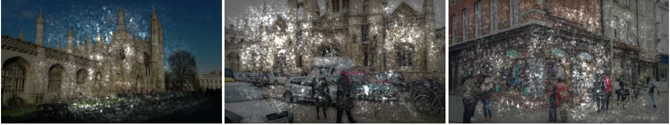
Figure 11: Saliency maps. This figure shows the saliency map superimposed on the input image. The saliency maps suggest that the convnet exploits not only distinctive point features (à la SIFT), but also large textureless patches, which can be as informative, if not more so, to the pose. This, combined with a tendency to disregard dynamic objects such as pedestrians, enables it to perform well under challenging circumstances. (Best viewed electronically.)
