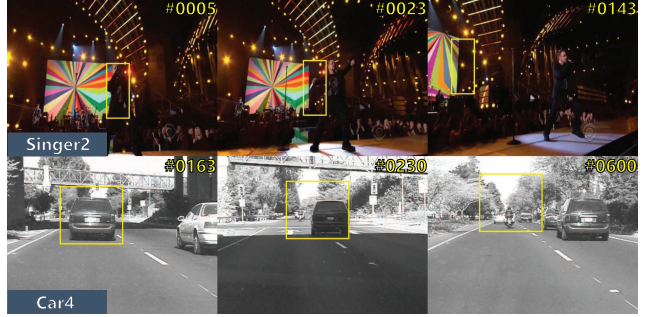
Figure 2. Inclusion of background information within an object bounding box due to complex object shape and size variation. In each of these sequence, background information causes a drift problem, and a tracker loses the target object eventually.
