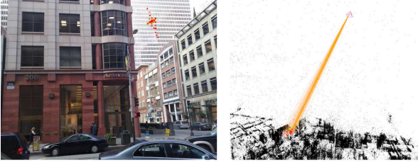
Figure 3: A sample query image with a pose that has more than 30 inliers even though it is obviously wrong. Inliers are only found in a small region of the image, forcing pose estimation to place the camera far away from the scene. Note that structure-based localization approaches typically use a threshold of 12 inliers to detect bad poses.
