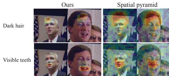
Figure 6. Spatial extent of attributes discovered by our approach vs. a spatial pyramid baseline. Red/blue indicates strong/weak attribute relevance. Spatial pyramid uses a fixed rigid grid (here 20x20), and so cannot deal with translation and scale changes of the attribute across images. Our approach is translation and scale invariant, and so its discoveries are much more precise.
