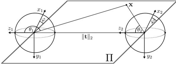
Figure 2: **Spherical Rectification.** Given two fisheye cameras  $(x_1, y_1, z_1)$  and  $(x_2, y_2, z_2)$ , we rectify the images yielding an angular representation  $(\theta, \varphi)$  where pixels in the same row (i.e., same  $\varphi$ ) are located on an epipolar plane  $\Pi$ .
