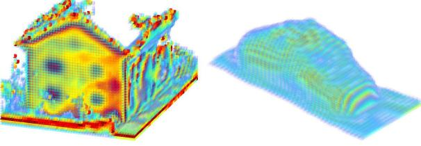
Figure 3: **Visualization of TSDF Model.** This figure shows a volumetric visualization of the learned TSDF model mean for a building (left) and a car (right). Red colors indicate voxels close to the estimated surface (i.e., 0-level set)
