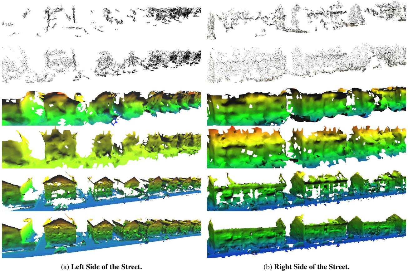
Figure 8: **Qualitative Results.** This figure shows our reconstruction results from both sides of the same street, respectively. From top-to-bottom: Point cloud from PMVS2 using the default parameter setting, point cloud from PMVS2 with optimized parameters, PMVS2 (optimized) + Poisson, PMVS2 (optimized) + SSD, our initial reconstruction, and our fused result (PC 0). Note how our method is able to recover cars as well as missing building walls, and handling different types of buildings.
