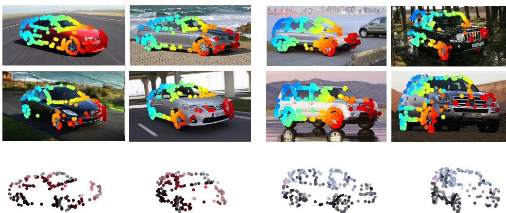
Figure 6. Matching different cars. Best viewed in color. Left: the correspondences of sedan images and the reconstruction. Right: the correspondences of SUV images and the reconstruction. Only four selected images are shown for each image set. Note that the cars in images are all different and the feature points are automatically detected. The markers with the same color indicate the matched feature points. The 3D reconstruction is rendered with the colors in the first image and visualized in two viewpoints.
