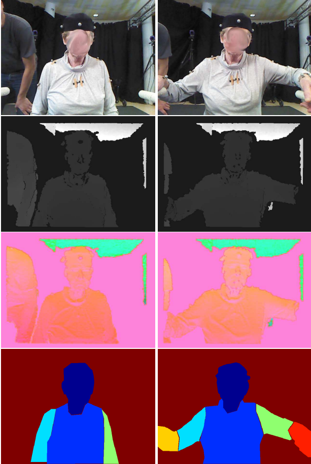
Figure 4. Example images from the dataset. Row 1 shows the RGB images. Row 2 shows the depth images. Row 3 shows the depth images encoded to 3 channel HHA [13], and Row 4 shows the pixelwise ground truth class labels.
