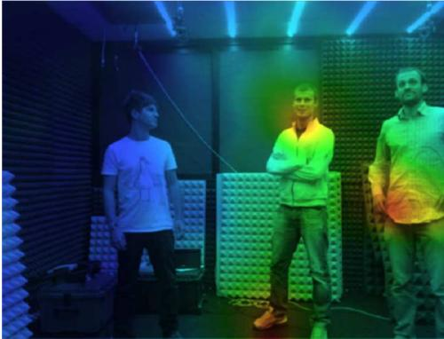
Figure 5. An example of audio/video frame extracted from the voice-sequence. In the acoustic map are visible the target sound (the voice) and some other sounds generated by the people movement.
