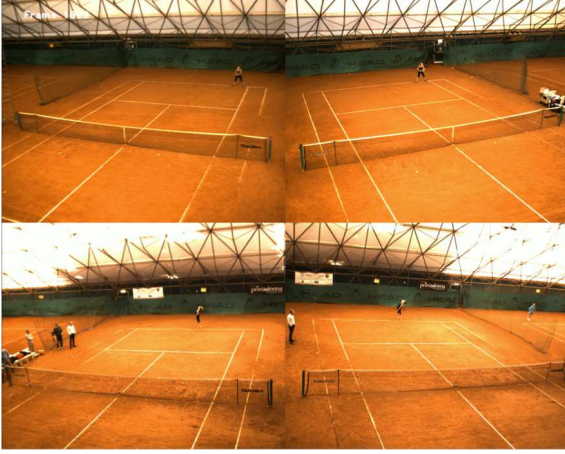
Figure 2. Example of synchronized acquisition. Four frames are captured exactly at the same time to make the system capable of observing the whole court from at least two different points of view.
