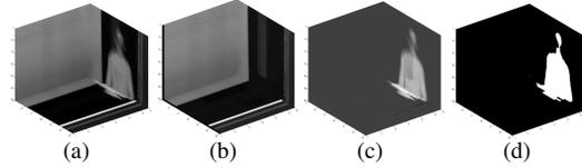
Figure 1: An example of tensor decomposition: (a) input, (b) *low-rank*, (c) *sparse* tensor, and (d) foreground mask.
