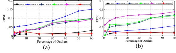
Figure 2: Performance of reconstructed *low-rank* tensor. (a)  $O = \max(\text{vec}(\mathcal{L}))$ , and (b)  $O = 10 \cdot \text{std}(\text{vec}(\mathcal{L}))$ .
