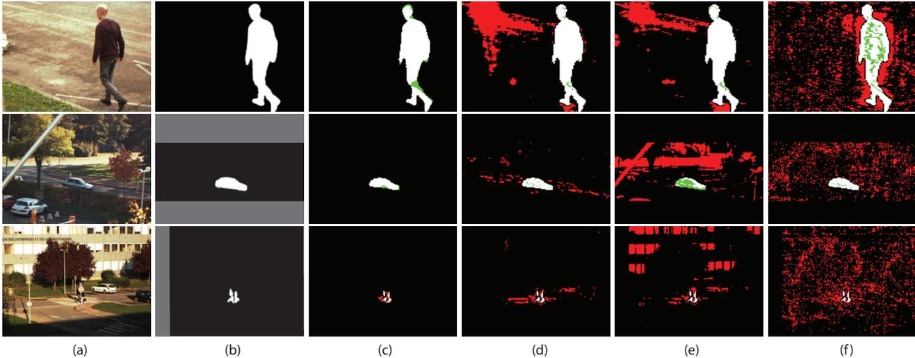
Figure 5: Visual comparison of background subtraction results over three scenes of the MSVS data set [1]. From left to right: (a) input image, (b) ground truth, (c) proposed approach, (d) BRTF [29], (e) HORPCA [7], and (f) CP-ALS [15]. The true positives ( $TP$ ) pixels are in white, true negatives ( $TN$ ) pixels in black, false positives ( $FP$ ) pixels in red and false negatives ( $FN$ ) pixels in green.
