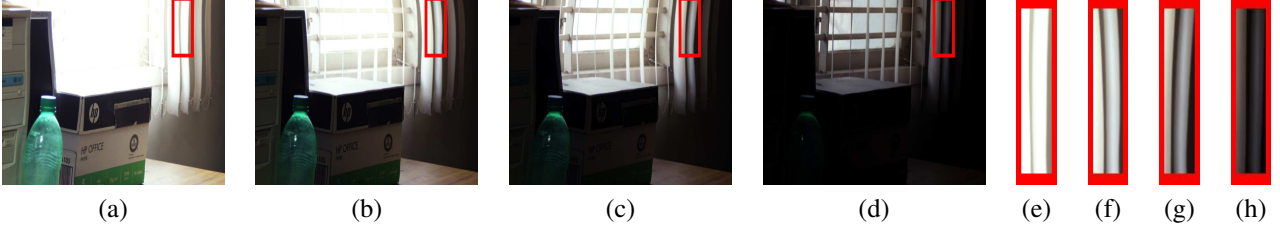
Figure 1. Multiple exposure frames affected by rolling shutter effect.
