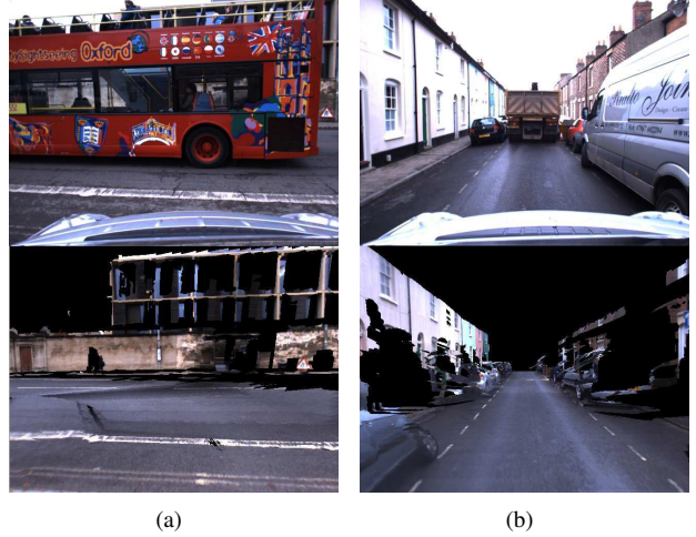
Figure 11. Failed localisation due to occlusions. (a) shows the field of view almost entirely occluded by a bus, and (b) shows a narrow street with many occluding vehicles and differences in parked cars. These cases could be resolved with a higher-level classification layer to detect and ignore dynamic objects for the purposes of localisation.
