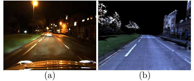
Figure 12. Failed localisation between a night-time dataset (a) and daytime prior (b). The localisation failed to converge for all images collected at night, due to the highly non-uniform illumination. A possible solution is a separate appearance prior collected at night, but this doubles storage requirements.
