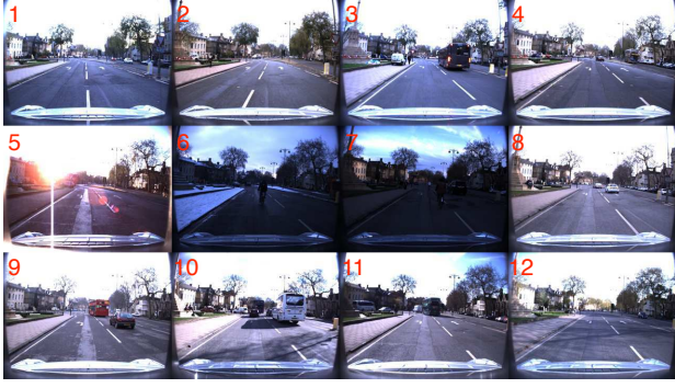
Figure 7. Camera images from a sample location for all twelve evaluation datasets. The traversals include significant variation in lighting and weather, including direct sunlight in dataset 5, snow in dataset 6 and seasonal vegetation change in dataset 9. Dataset 1 is used to build the scene prior; all subsequent datasets are matched to dataset 1.
