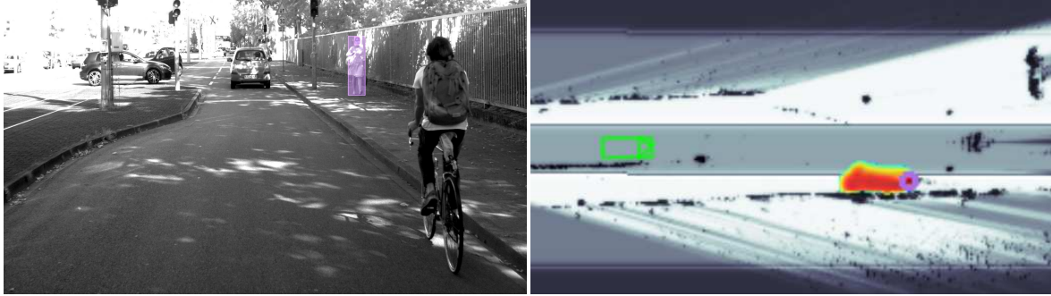
(a) Prediction of pedestrian on sidewalk. Possibility of stepping on the street is still tracked in Particle Filter, passing through the fence is excluded from path possibilities.
