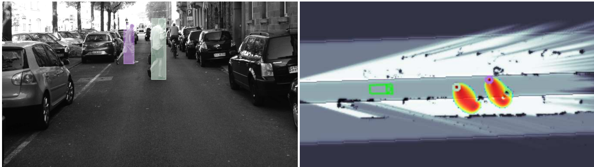
(c) Prediction of pedestrians crossing. Future walking direction on sidewalk is correctly inferred.
