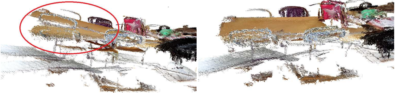
Figure 5. 3D reconstruction of a table using visual measurements only (left) and fusing inertial and visual measurements (right).
