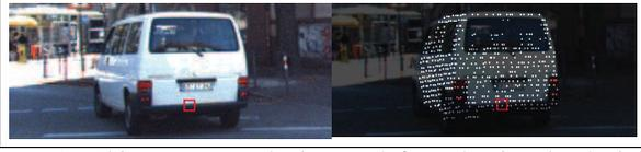
Figure 1. This paper uses the image (left) and point cloud (right) sources to reconstruct the surface.
