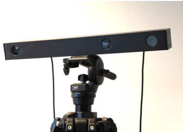
Figure 1. Our customized trinocular stereo camera setup with a baseline of  $40\text{cm}$  (between the left and right cameras). A commercially available alternative (no affiliation) can be found at [5].
