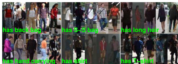
Figure 5. Some samples that are difficult to be classified in the binary attribute classification, when using AdaBoost classifiers and fusion features. Many incorrectly classified S-S bag and back bag samples have only the sash parts appearing. Results are affected by similar clothing color appearing on shoulder region ( long hair ), occlusion ( hand carrying ) and weak illumination ( shirt and T-shirt ).
