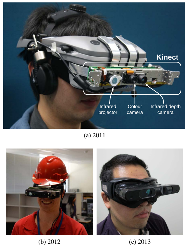
Figure 8: Wearable Computer Vision Systems (HMD) for Simulated Prosthetic Vision developed by MVG.
