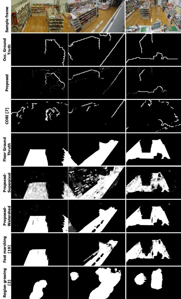
Figure 8: Experimental result for static occlusion boundary likelihood estimation and floor likelihood estimation (see text for discussion).
