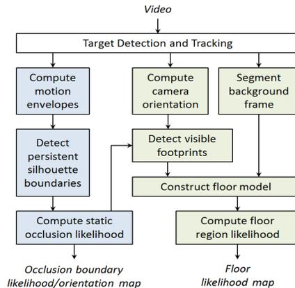
Figure 2: Proposed framework for scene geometry estimation.
