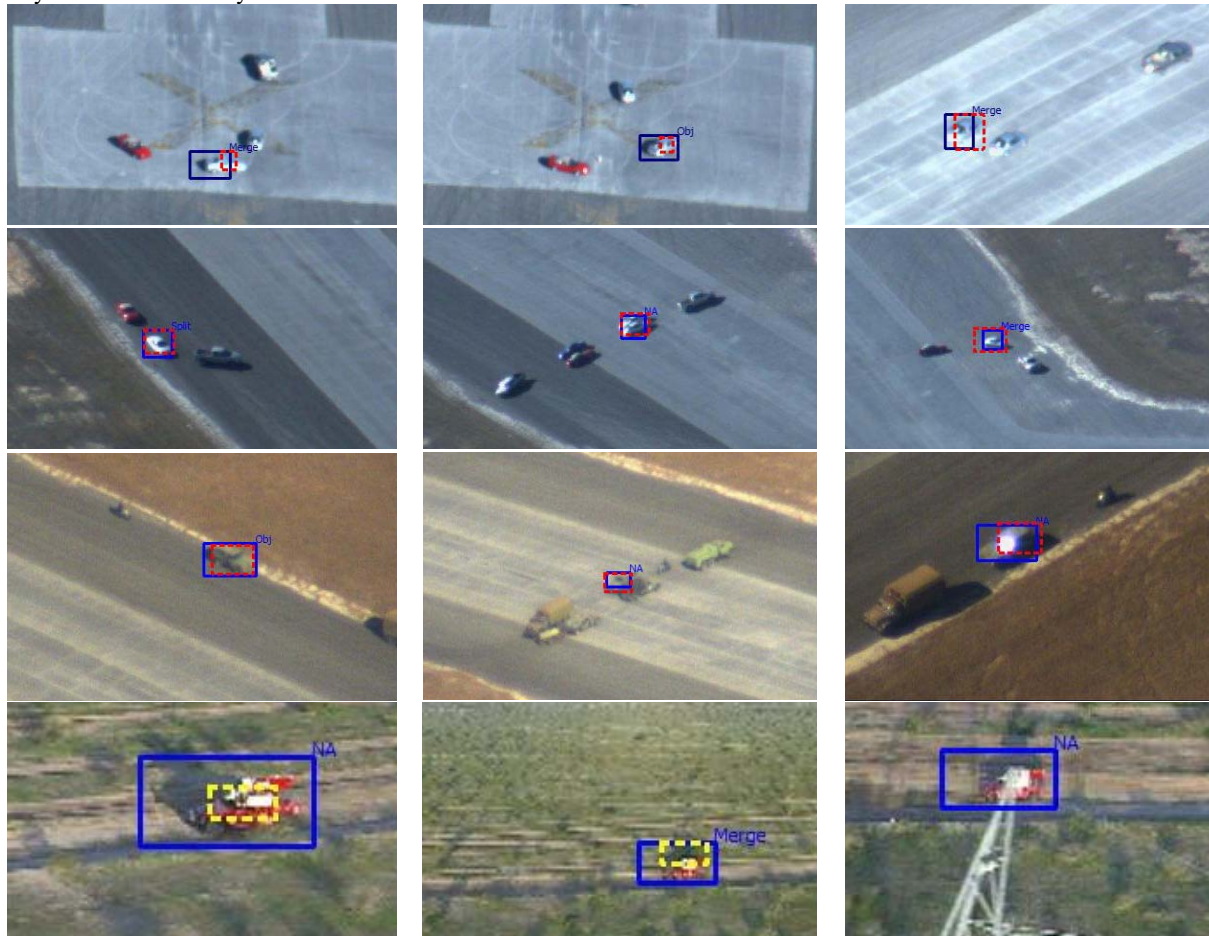
Figure 6: Qualitative Analysis, blue solid line is the proposed work, and the dashed line is the output of TLD. From top to bottom, the datasets presented are Eglin1, Eglin2, Eglin3, and Redteam. From left to right, Eglin1 Frame #301, 351, 1355. Eglin2 Frame # 301, 641, 848. Eglin3 Frame # 50, 561, 2457. Redteam Frame # 613, 780, 523.
