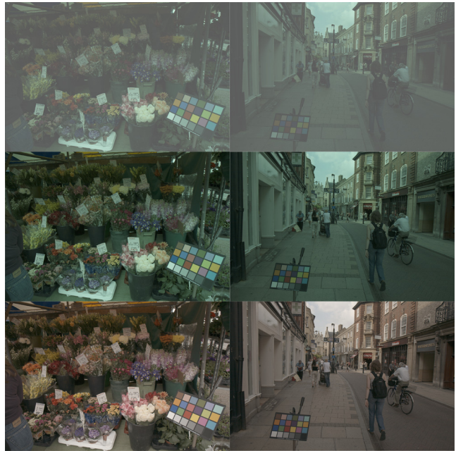
Figure 4. Top: The Shi and Funt reprocessing of the Gehler Dataset. Middle: Corrected Black Level. Bottom: Our Processing with Black Level Correction and D65 Colour Correction.
