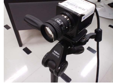
Figure 13. Polarization imaging camera.
