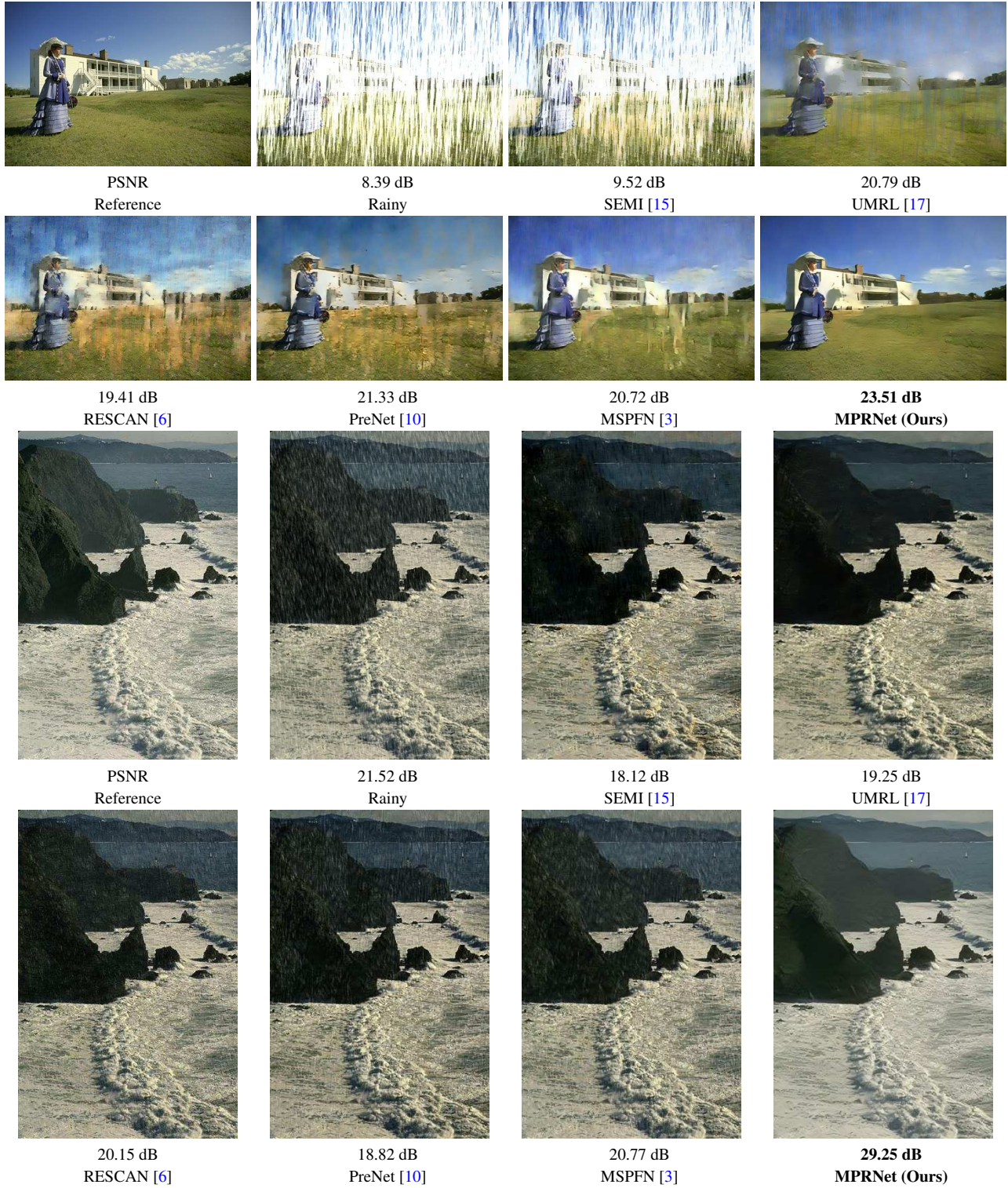
Figure 4: Visual examples for image deraining. Top image is from Rain100H [16], and the bottom is from Test100 [22].
