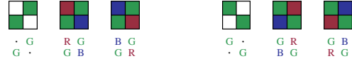
Figure 3: The four possible sampling patterns can be grouped by the diagonal on which the green channel was sampled: \begin{smallmatrix} R & G \\ G & B \end{smallmatrix} and \begin{smallmatrix} B & G \\ G & R \end{smallmatrix} share the \begin{smallmatrix} \cdot & G \\ G & \cdot \end{smallmatrix} diagonal, whereas \begin{smallmatrix} G & R \\ B & G \end{smallmatrix} and \begin{smallmatrix} G & B \\ R & G \end{smallmatrix} share the \begin{smallmatrix} G & \cdot \\ \cdot & G \end{smallmatrix} one.
