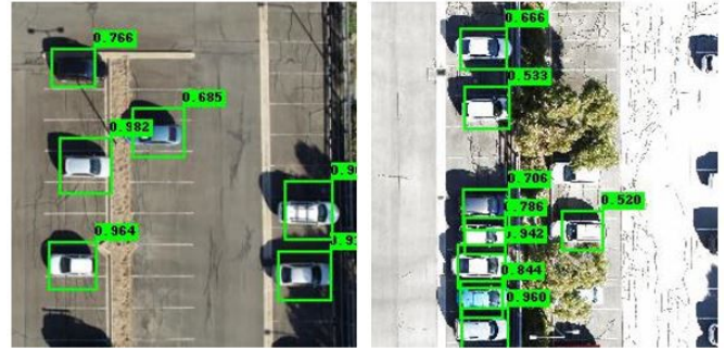
(a) No patches embedded in an original testing image (STD) and the weather (snow) augmented version of the testing image (STD-W).
