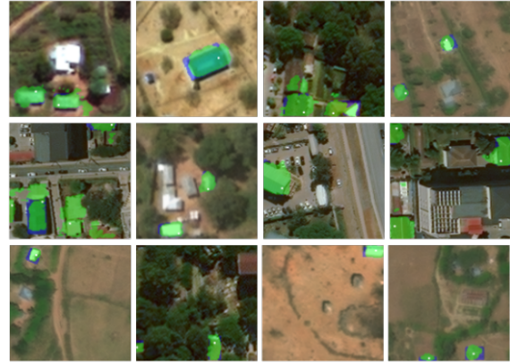
Figure 3. Sample segmentation outputs using an indicator point to specify which building(s) to segment[11]. White dots show input points given to the model to specify which buildings to segment. Green shows predictions and blue ground-truth.
