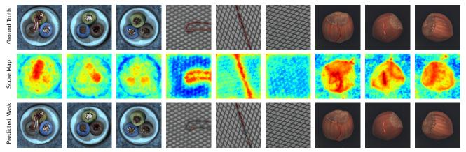
Figure 3. Examples of the input images with ground truth anomaly masks (top row) for various classes of the MVTec. Our CFLOW-AD model from Table 4 estimates anomaly score maps (middle row) and generates segmentation masks (bottom row) for a threshold selected to maximize F1-score. The predicted segmentation mask should match the corresponding ground truth as close as possible.
