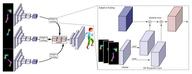
Figure 2: Our model processes keypoints which are split into individual layers. The resulting features for each keypoint layer are then scaled, concatenated, and used to generate the final image.
