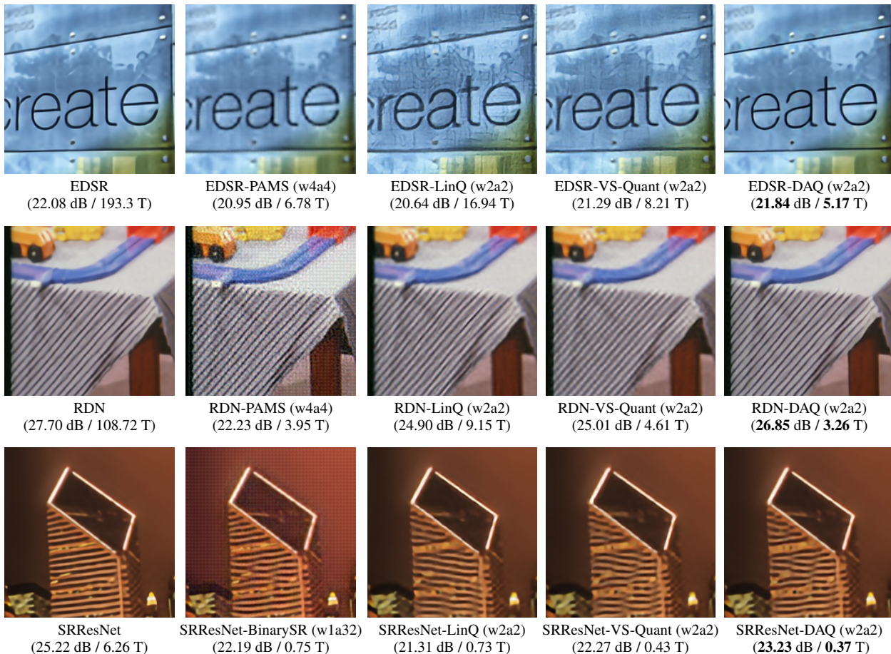
Figure 5: Qualitative evaluation of existing quantization methods on EDSR [32], RDN [48] and SRResNet [30] of scale 4, as in Figure 5. Evaluation is done on 'barbara' of Set14 and 'img060' and 'img097' of Urban100. Quantitative measures are also denoted (PSNR / BOPs).
