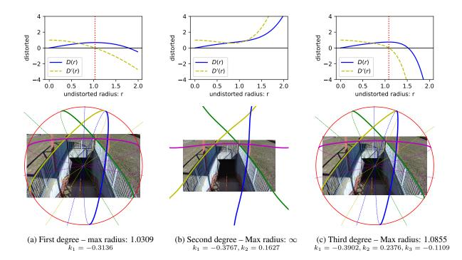
Figure 4: First through third degree Brown–Conrady distortion functions fit with OpenCV to the same data. Top: plots of D(r) and D'(r) for each case with the maximum valid radius marked in red. Bottom: multiple straight world lines distorted under each model. These fold at the maximum valid radius (red circle) in the first and third but not second degree case. All radius units are reported in the undistorted space.
