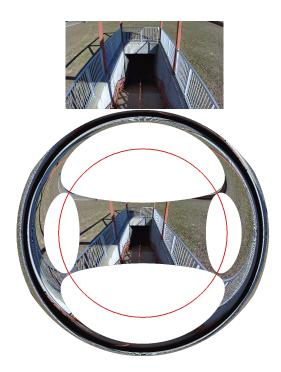
Figure 1: Example of undistortion. Beyond the red circle (maximum radius of distortion) the distortion folds back on itself. Points outside the maximum radius may incorrectly project into the valid image bounds causing problems in practical vision applications.
