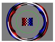
(c) Undistortion for a Sigma 14mm f/1.8 DG HSM | A. r<sub>normalized</sub> = 1.478 is shown in green.
