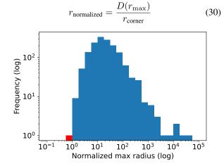
Figure 5: Histogram of normalized finite maximum radii,  $r_{\text{normalized}}$ , on a log-log plot. Only one model, corresponding to Figure 6b, has  $r_{\text{normalized}} < 1$ , meaning folding occurs within the bounds of the input distorted image. Note that most other models still have problematic distortion in the case of forward projection, as shown in Figure 2.
