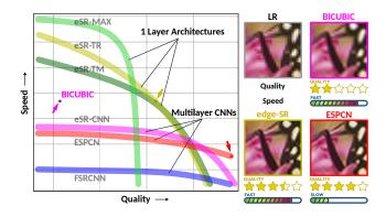
Figure 1. Trade–off pattern observed in our experiments. A standard upscaler (e.g. bicubic) is fast and can be deployed in any display hardware. Multilayer CNNs reach better quality but show sharp loss in quality when their size is reduce to make them faster. We propose edge–SR (eSR) one layer architectures that can adjust the size to reach the best possible quality for a display hardware.
