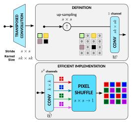
Figure 2. Classic  $s \times s$  image upscaling is performed by a transposed convolutional layer. An efficient implementation splits the filter into  $s^2$  smaller filters that work at LR. The final output is obtained by multiplexing the  $s^2$  channels using a pixel–shuffle layer.
