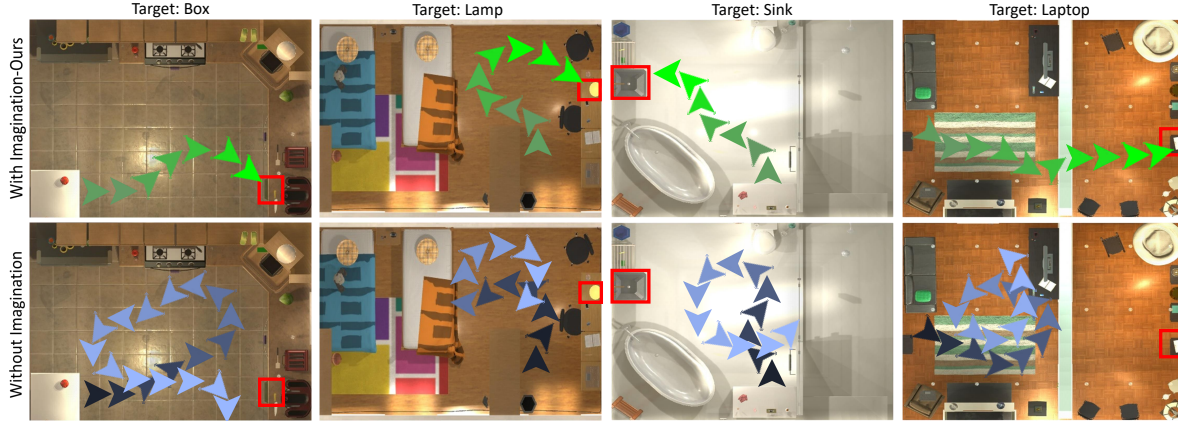
Figure 3. Qualitative comparison of navigation episodes of ForeSI against the baseline method [39] in four different room types. The examples represent cases where our method improves both the robustness and the efficiency of navigation. For more examples and failure refer to supplementary material.
