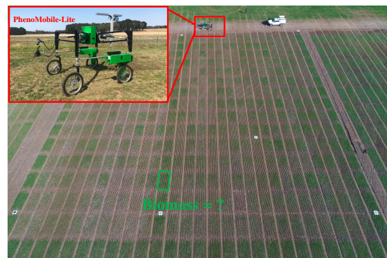
Figure 1. Overview of fields. Our method aims to predict the biomass of each plot via the scanned point cloud. The point cloud is obtained by the PhenoMobile-Lite ® (zoom-in of the red box). (Best viewed in colour on screen.)
