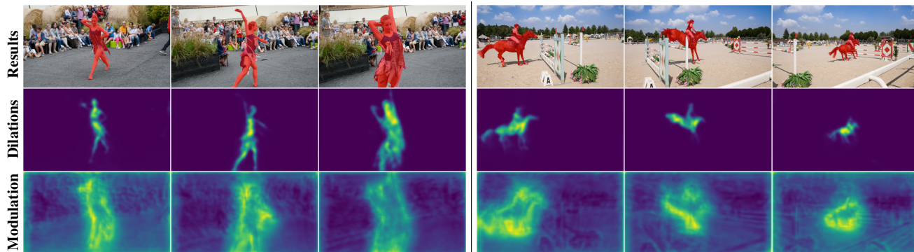
Figure 4: Qualitative results on DAVIS’16 [25]. Depicted are results from our model (top row), mean predicted dilation factors (middle row), and mean predicted modulation values. Lighter pixels denote higher values. Dilation factors are highest on the object, while modulation values are highest on the object boundary. Left sequence is dance-twirl , right sequence is horsejump-high .
