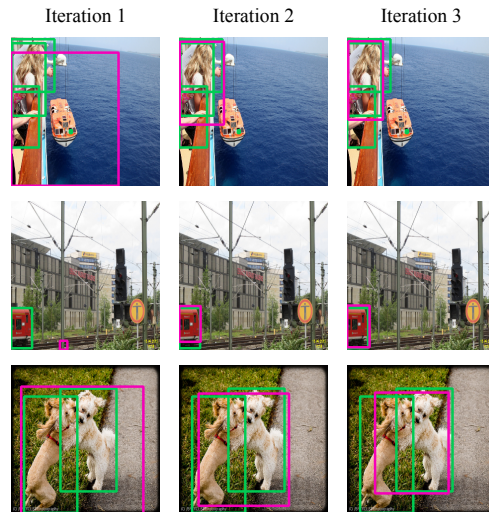
Figure 6. Bounding box adjustments at each iteration for the common object localization experiment on COCO60 with K = 5 . Only the top prediction in the query image is shown (in pink color) for each iteration. Ground-truth bounding boxes of the target classes are shown in green. EM refinements improve the target object localization in the query image.
