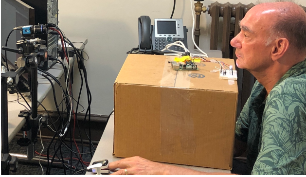
Figure 3: Image of the collection setting during a physical attack. The attack device is placed just below the subject’s chin out of the camera’s frame.
