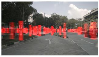
Figure 1. Visualization of the camera image, augmented with the uncertainty weighted RCS channel values highlighted in red.
