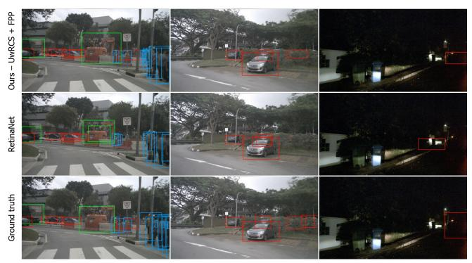
Figure 3. Qualitative comparison of detection results. Red: Car, Green: Truck, Blue: Pedestrian.
