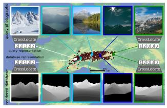
Figure 1. **CrossLocate** localizes ground-level photographs captured in diverse environments across the Alps. Our new databases of rendered image modalities enable the implementation of crossmodal image-retrieval (*i.e.* matching real photographs to rendered imagery). Out of several assessed modalities, we select depth maps and train a cross-modal global descriptor for large-scale image localization outdoors.
