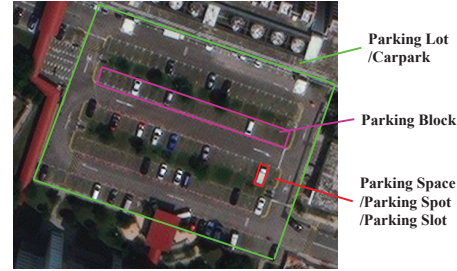
Figure 2: Illustrations of parking lot, block, and space. Original Image © 2018 Maxar Technologies Inc.
