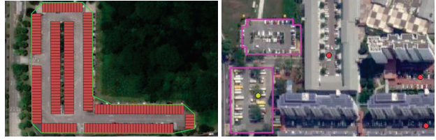
Figure 5: Left: parking slots are grouped based on locations to form the polygon candidates. Right: only the points ( i.e. , red dots) that are not covered by any polygon candidates ( i.e. , pink polygons) are kept for further labeling. Those already been covered ( i.e. , yellow dots) are discarded. Original Images © 2018 Maxar Technologies Inc.
