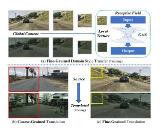
**Figure 6:** We optimize CycleGAN with receptive field restrictions to conduct detection-oriented fine-grained style transfer.
