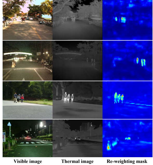
Figure 4. Visualization of the visible-thermal image pairs and the 2-D spatial re-weighting masks from the proposed F-MSE loss. The first two lines of multispectral images pairs come from KAIST Dataset, and the last two lines come from MFNet Dataset.
