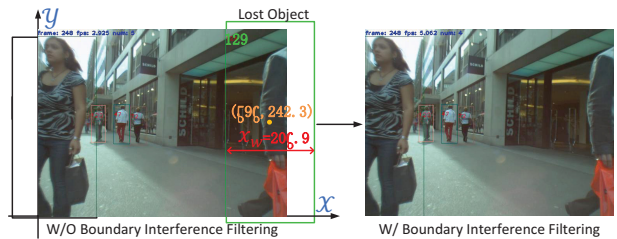
Figure 5. Diagram of boundary interference filtering result. The width and height of the image are 640 and 480 respectively. The center coordinate of the lost object 129 is (596, 242.3) and its width x_w is 206.9. Because the object 129 does not satisfy the formula (8), it will be filtered out.
